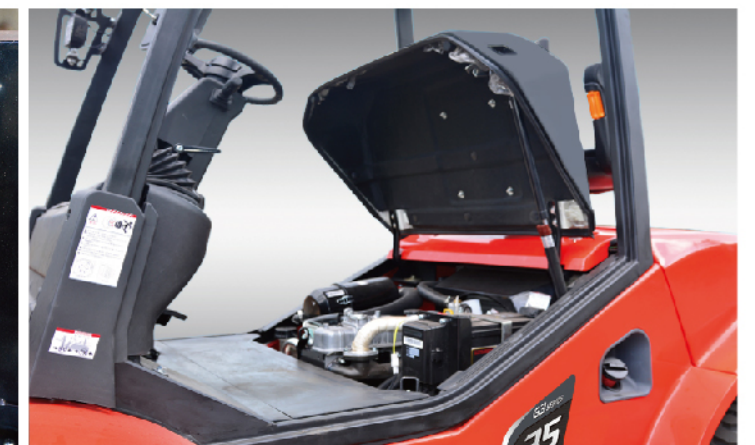
Engine cover with large opening angle, large maintenance space
