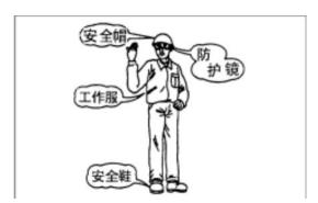
Please wear proper safety clothes when driving. Improper clothes may be caught by operating levers or pedal which may cause truck mis-moving.
