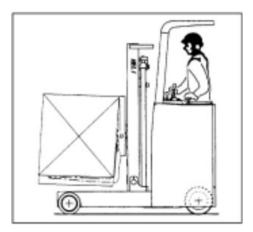
The main use of reach truck is handle and stack the loads that on the pallets. When they are assembled with proper attachments, they also can handle the loads that not on the pallets.
