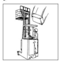
The overhead guard is used to protect the driver when goods are falling from the top of head. But it does not mean it can withstand the impact of all falling goods.
