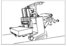
(12) When travelling backward, it is dangerous to depend on back view mirror only. Face backward and travel after a direct check of the backward.
